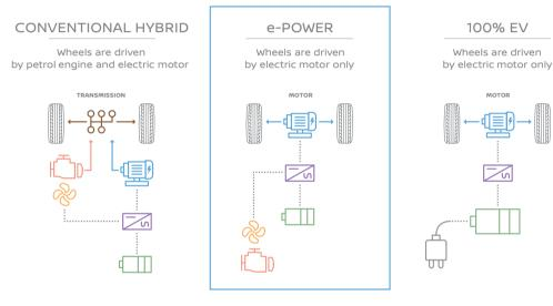
ENGINE GENERATOR BATTERY ELECTRIC MOTOR INVERTER
